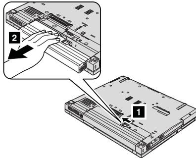
4. Install a fully charged battery.
