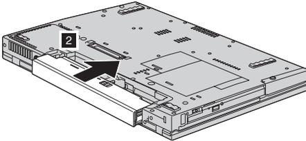
5. Slide the battery latch to the locked position.
