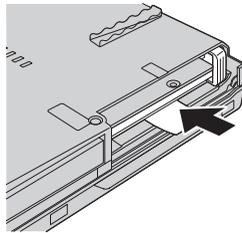
10. Reinstall the cover of the hard disk drive slot.
