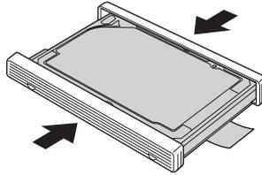
9. Insert the hard disk drive into the hard disk drive bay; then press it firmly in to place.
